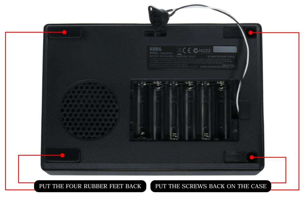
9.1 - Using a Phillips screw driver, put the screws back on the case 9.2 - Put the four rubber feet back
